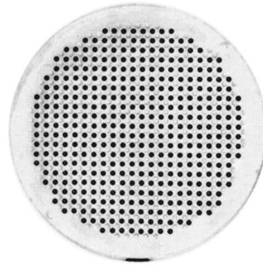
FIG. 2. Photograph of a typical periodic specimen containing steel particles with  $A_f=0.32$ ,  $d=2.63$  mm, and  $a=0.58$  mm.
