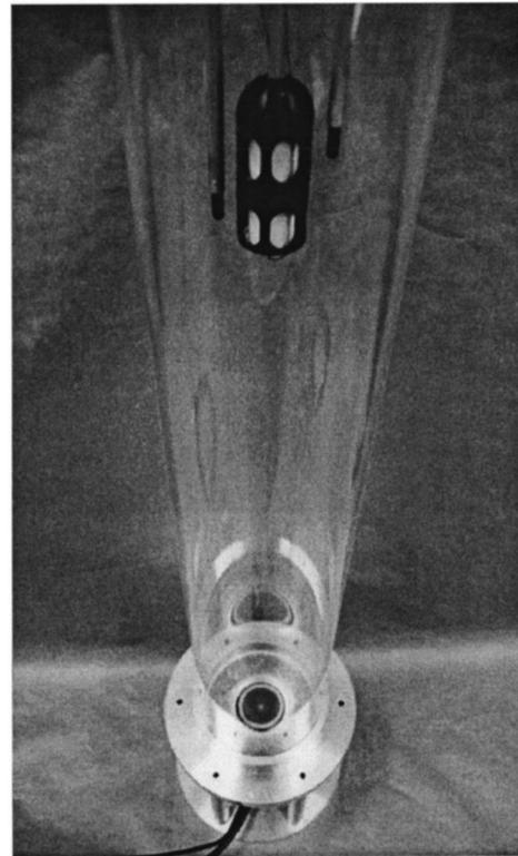
FIG. 4. The slow wave calibrator with the *u-u* intensity probe and reference transducers suspended from above. Note that the two cables attached to the USRD J9 source are for the electrical driving signal and the driver's hydrostatic pressure compensation.
